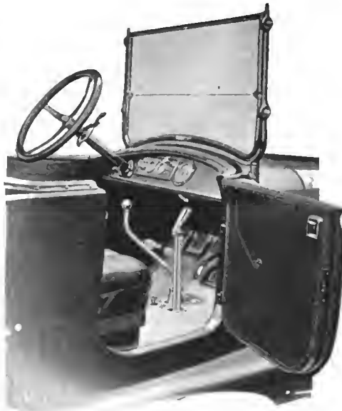
Driver's compartment of the 1917 Grant, showing the wide door and the arrangement of the control levers. Note the simplified instrument board
